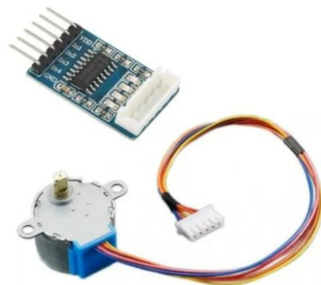
Figure 15. Stepper motor used to drive the lead screw [15]
